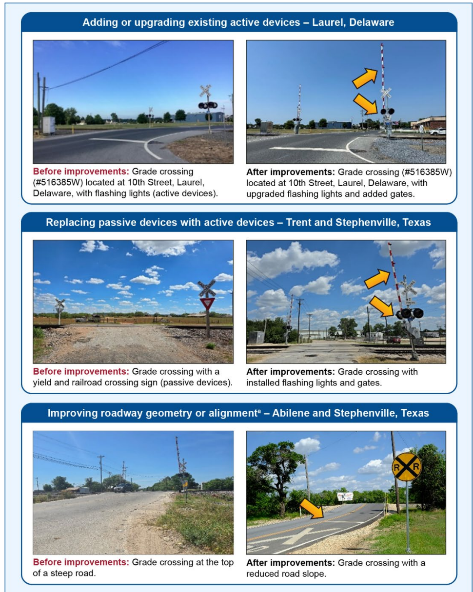
Figure 1: Examples of Railway-Highway Crossings Program Project Types, Before and After Improvements
