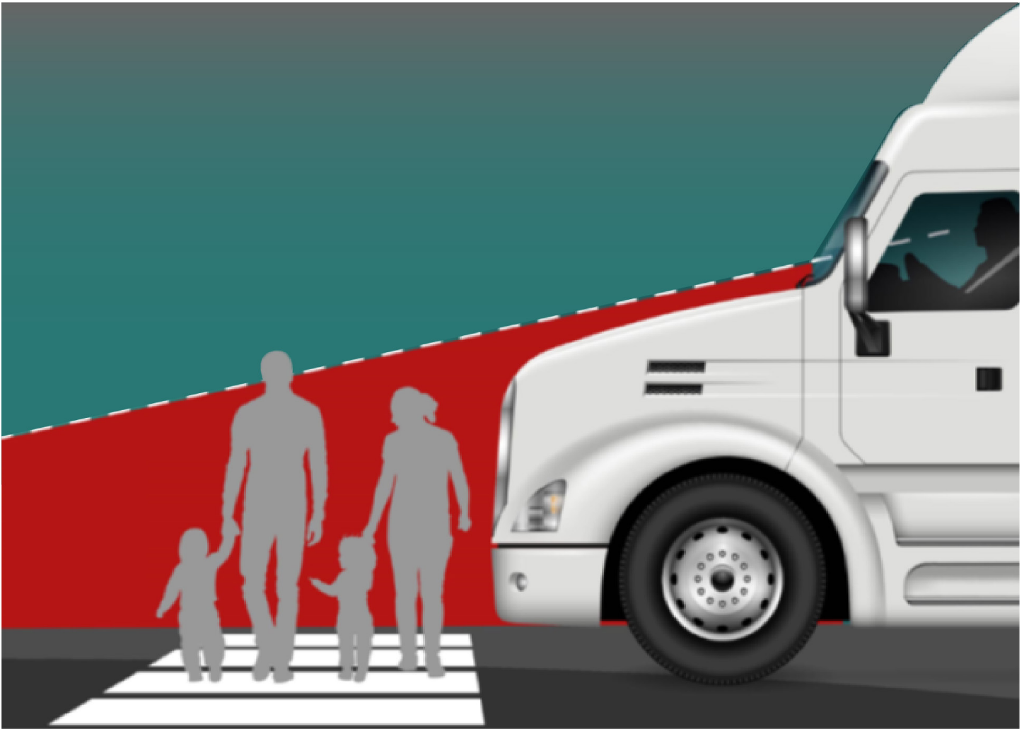
Figure 4: Department of Transportation Example of a Possible Front Blind Zone in a Commercial Truck
