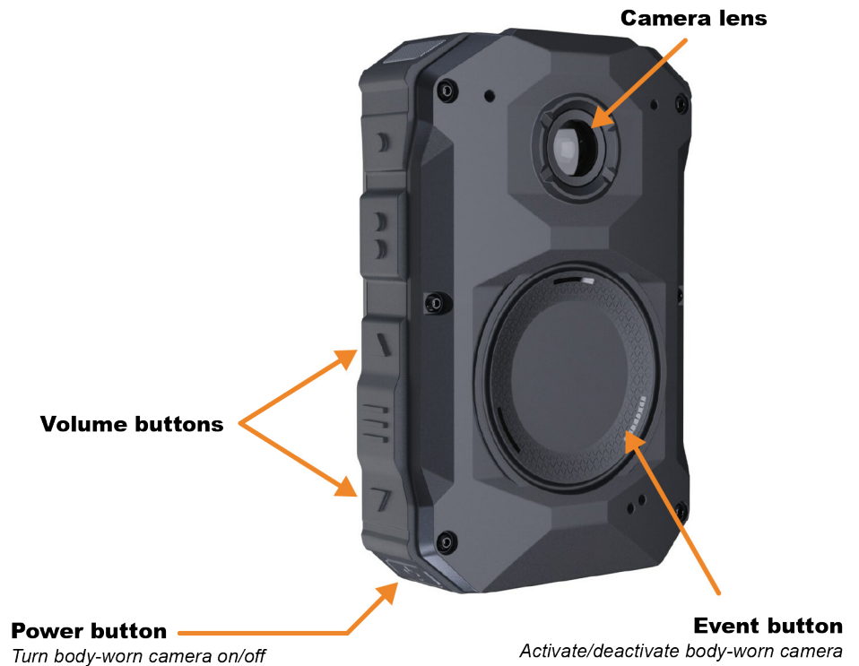
Figure 1: Body-Worn Camera and Functional Buttons
