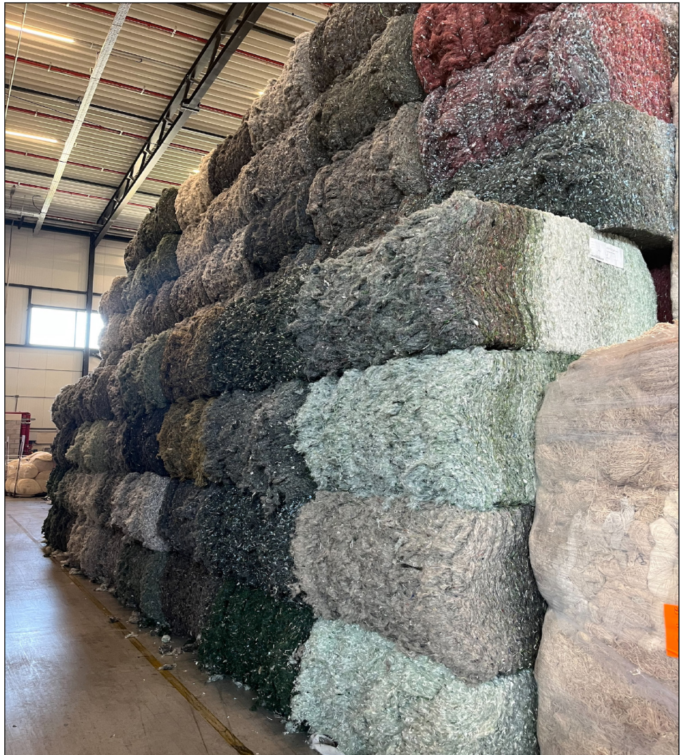
Figure 5: Example of Mechanically Shredded Textiles at a Textile Recycling Facility
